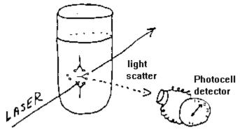
Mix patient's serum with antibody to the component of interest, and immediately shine the laser through the tube (all done automatically).
